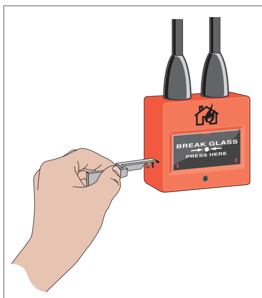
Figure 4: Sketch of fire alarm frangible cover break
