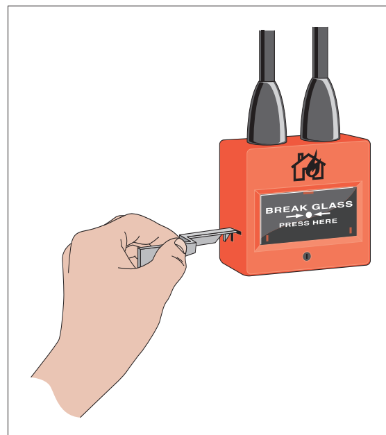
Figure 19: Using a test key
